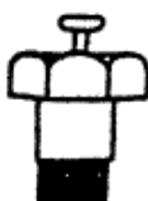
HAMMER HEAD BOLT. FOR HARD TO START HOLES
