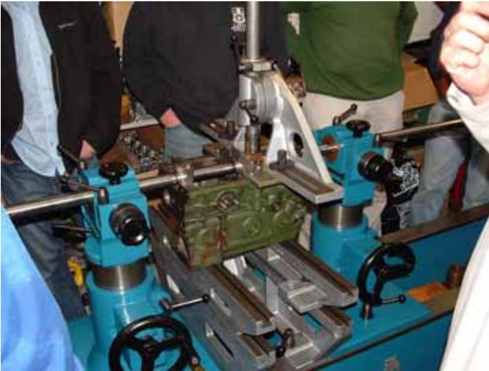
*Machining an A series block*
