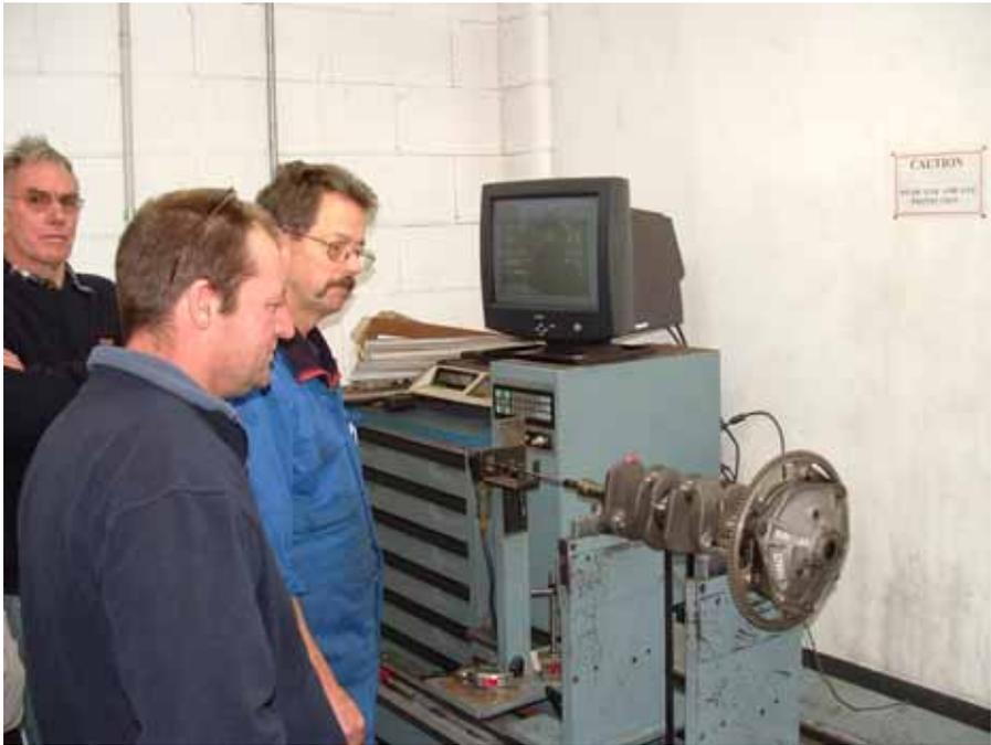
*Balancing a Mini crankshaft & flywheel*
