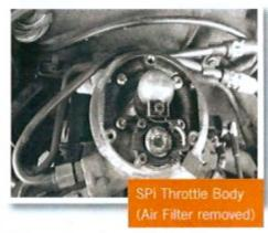
If the car has air-conditioning it's probably a JDM import. Firstly check the plastic oval shaped air filter for the injection wording moulded into the top. The ECU should be on the left of the engine bay when viewed from the front. Under the air filter to the left hand side there are two metal fuel feed and return
