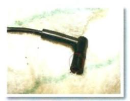
On the SPi Mini's you'll find four of these, they have right angle rubber ends and a flexible plastic capillary tube linking them. There are two that run from the Inlet manifold, one to the ECU computer MAP sensor via a fuel trap and the other to the base of the air filter enclosure with a third running to the hot air valve. If any of these are loose, missing or cracked a false reading will be fed to the computer resulting in a difference fuel / air mixture based on engine load and speed.
