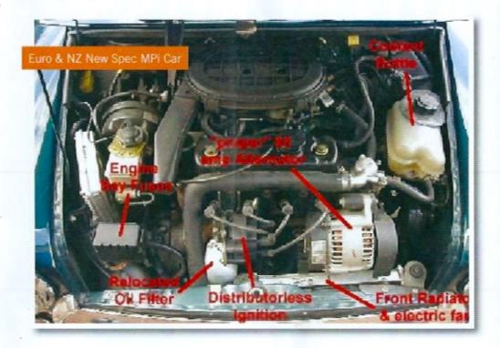
Euro spec and NZ new MPi cars have the same plastic air filter casing but will have a front mounted radiator, expansion bottle, Oil filter mounted directly onto the block, coil pack and two injectors on top of the inlet manifold directly before the inlet port. The ECU is of a smaller design and the MAP sensor is fitted directly to the inlet manifold with an electrical signal fed to the ECU deleting the need for the troublesome vacuum capillary pipes.
