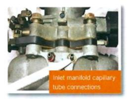
Access to the reverse of the inlet manifold is severely limited, once the three bolts securing the air cleaner are removed then it can be lifted from the throttle body. Remove the capillary tube from the air cleaners base and place the cleaner to one side. You will now be able to reach down the back of the throttle body and feel your way to locate the two capillary pipe connections on the rear of the manifold. Simply pull these off noting the order, left to right on their location.
